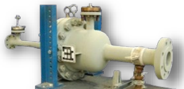
5 MWth Natural Gas CPOX
