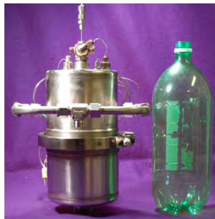
Figure 3: Photo of the 5\text{ kW}_{th} reformer prototype hardware (inclusive of steam generator, fuel/air/steam premixer, atomizer, igniter, sulfur cleanup).
