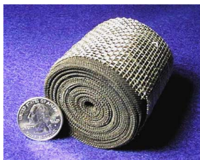
Fig. 3. Radial flow Microlith reactor for oxidative steam reforming of methanol.
